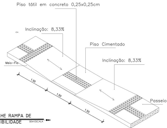
DETALHE RAMPA DE ACESSIBILIDADE SEM ESCALA
