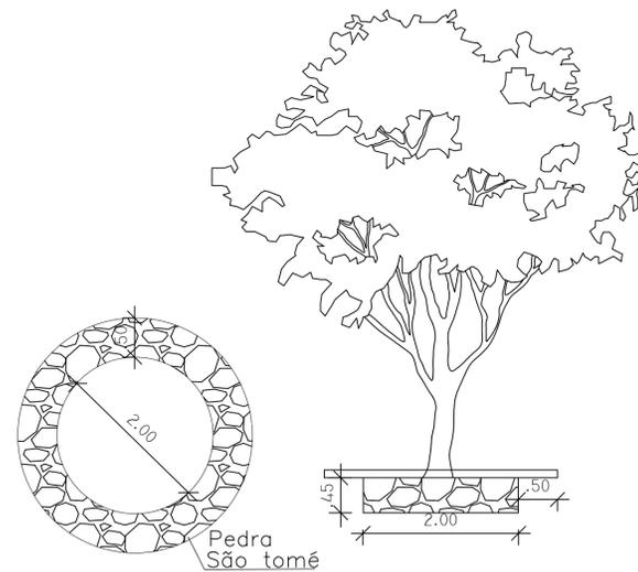
DETALHE DA ALVENARIA DA ÁRVORE SEM ESCALA
